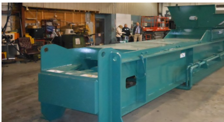
Harris badger LSOS baler in place at the Roane County Recycling Hub.
